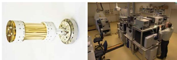
The Center is uniquely equipped with several Fourier-transform mass spectrometers, including the new dynamically harmonized analyser cell (left) dramatically increasing resolving power.
